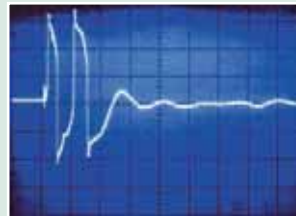
Oscilloscope reveals harmful high frequency transients at the output of conventional power protection products.
