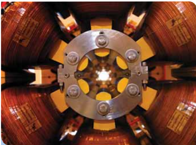
One of the 48 bending magnets used to maintain the 3GeV electron beams.
